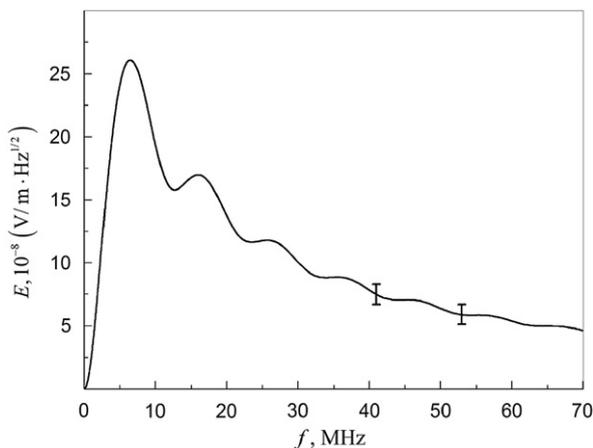
Fig. 5. Spectrum of electromagnetic radiation at distance 300 km from the epicenter. The vertical sections of line denote the experimental data. The following parameters are chosen for calculations:  $I_0 = 50$  A,  $\nu = 2 \times 10^5$  s $^{-1}$ ,  $u = 10^8$  m/s,  $\tau = 10^{-7}$  s,  $\alpha = 2 \times 10^7$  s $^{-1}$ ,  $\beta = 8 \times 10^7$  s $^{-1}$ ,  $d = 40$  km,  $h = 1$  km,  $z_0 = 6$  km.
