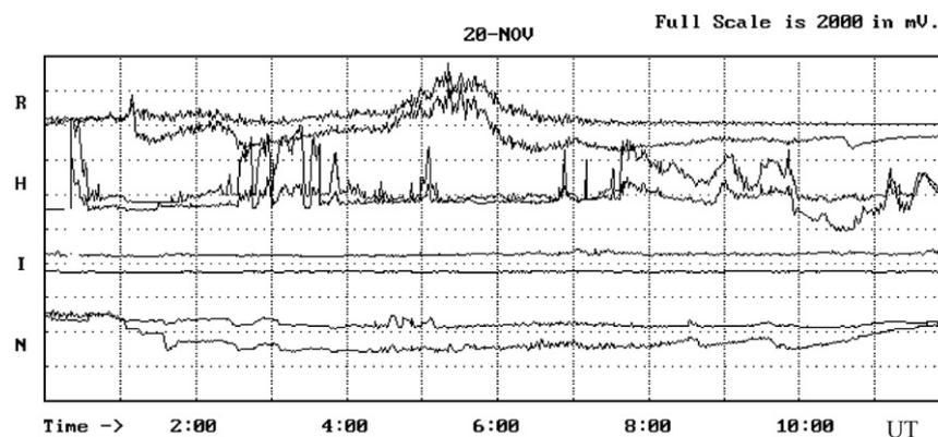
Fig. 1. The pre-seismic VHF signals for the November 21, 1992 EQ ( $M=6.0$ ). The output voltage of the receivers presented is given on the vertical axis. Full scale is 2000 mV (Ruzhin and Nomicos, 2007). N, I, H and D represent the observing stations of Nipos, Ierapetra, Heraklio and Drapania, respectively, forming Crete monitoring station.
