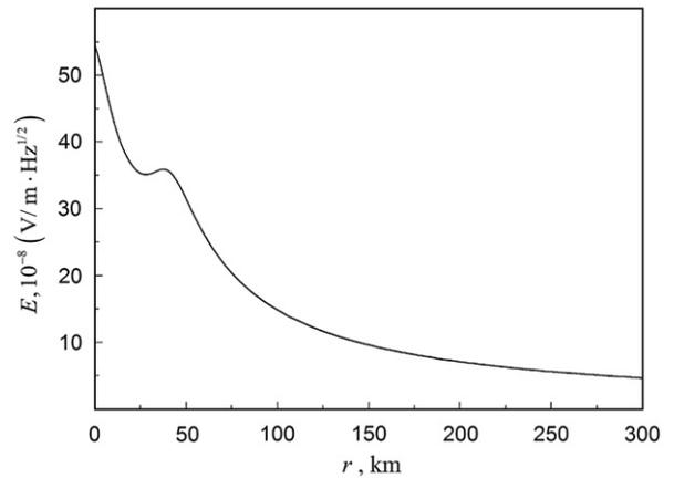
Fig. 6. Dependence on distance of the amplitude of electromagnetic radiation at a frequency 50 MHz. The following parameters are chosen for calculations:  $I_0 = 50$  A,  $\nu = 2 \times 10^5$  s $^{-1}$ ,  $u = 10^8$  m/s,  $\tau = 10^{-7}$  s,  $\alpha = 2 \times 10^7$  s $^{-1}$ ,  $\beta = 8 \times 10^7$  s $^{-1}$ ,  $d = 40$  km,  $h = 1$  km,  $z_0 = 6$  km.
