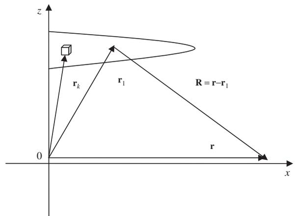
**Fig. 4.** Coordinates used for the calculation of characteristics of electromagnetic radiation.
