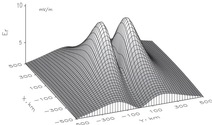
Fig. 2. Calculation results of the spatial distribution of radial component of electric field in the ionosphere (Sorokin et al., 2006).
